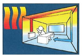
Transfer of thermal energy using moving air as transfer fluid between the heating system and the persons to be heated. The air temperature is always greater than the temperature of the walls of the room heated.
