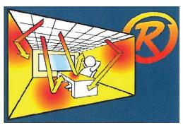
Transfer of thermal energy using infrared waves as a transfer vector between the heating system and the rooms and/ or persons to be heated. The air tempera-
