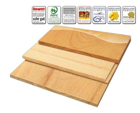
Due to the 3-layered-construction, the highest possible dimensional stability is gained. Compared to a traditional solid wood board, shrinkage and swelling is minimized by up to 70 %. For gluing, we only apply glue of the strain-group D3 (moist-solid) according to EN204. Caused by production, it might be possible that some boards have a middle layer in a different sort of hardwood, which - in no way - affects the quality of the parquet.
